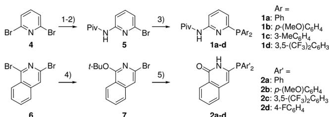
**Scheme 2:** Synthesis of monodentate aminopyridines **1** and isoquinolones **2**: 1) NH<sub>4</sub>OH, 190 °C, 5 h; 2) pivaloylchloride, NEt<sub>3</sub>, CH<sub>2</sub>Cl<sub>2</sub>, 0 °C → RT; 3) *n*-BuLi (2 equiv), THF, –100 °C, then ClPR<sub>2</sub>, –100 °C → RT; 4) KO<sup>t</sup>Bu (1.1 equiv), toluene, 80 °C, 1 h; 5) *n*-BuLi (1 equiv), THF, –100 °C, then ClPR<sub>2</sub>, –100 °C → RT, then H<sub>2</sub>O (1 equiv) and formic acid excess (50–75%).
