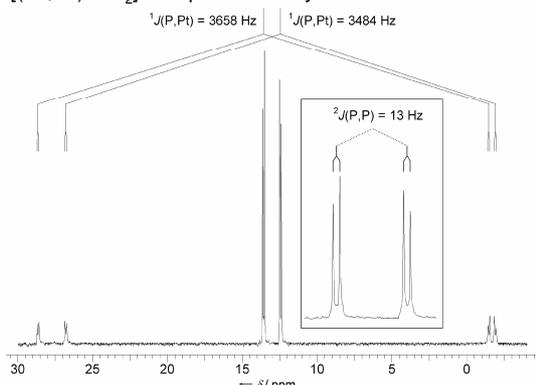
**Figure 1:** <sup>31</sup>P-NMR spectrum of *cis*-[(**1a,2a**)PtCl<sub>2</sub>] in CDCl<sub>3</sub> solution.
